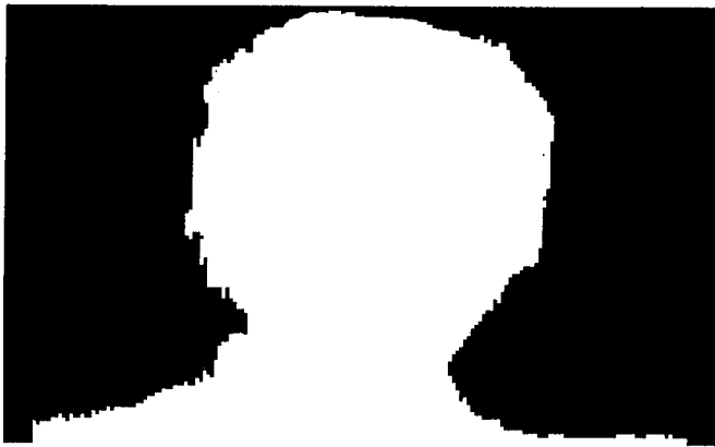
Figures 12, 13: Depth-from-focus data can be used to create a key mask (left) for placing a figure against a different background (right).
