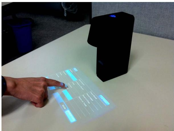
**Fig. 4.** Holographic projector combined with infrared touch sensor, used in an interactive restaurant menu application. Courtesy of Light Blue Optics Inc.
