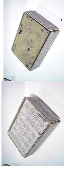
**figure 2.** The Bar of Soap V1 prototype with (a) back side up and (b) front, sensor-less side up.
