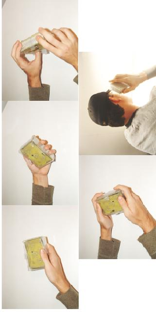
**figure 3.** The Bar of Soap held in five poses: remote control, PDA, camera, game controller and phone. Note that other grasps were used by subjects in the tests.
