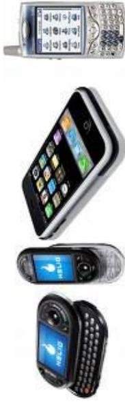
**figure 1.** Commercially available multi-function handheld devices. The Hello Ocean (A) employs a sliding screen that reveals different button sets. The Apple iPhone (B) uses virtual buttons on a touchscreen. The Palm Treo (C) has a touch screen in addition to a variety of physical buttons
