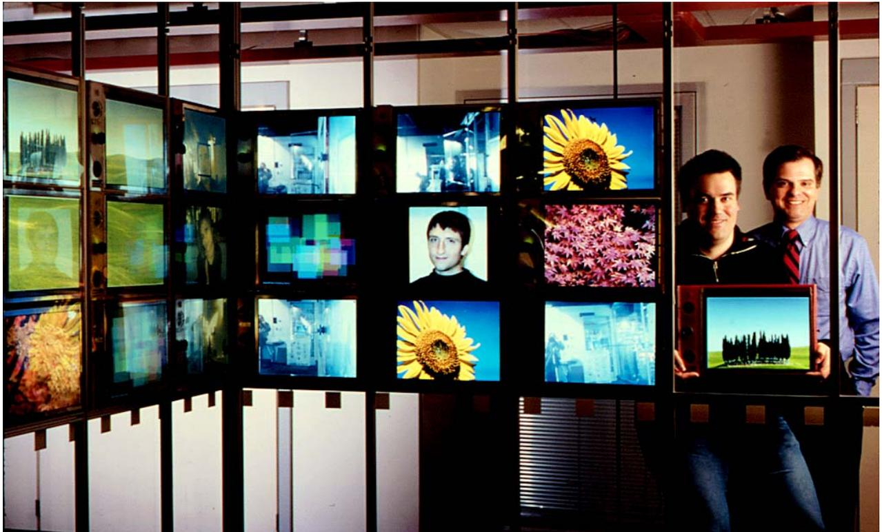
Fig 2 A set of Smart Architectural Surfaces tiles, each containing camera, display, speaker, microphone, and other sensors. [Photo credit: Webb Chappell]
