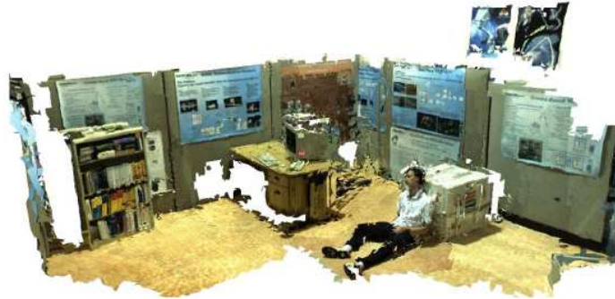
Figure 5-1: Figure from [Se and Jasiobedzki 2005] showing reconstructed scene with areas missing due to occlusion and matching error.
