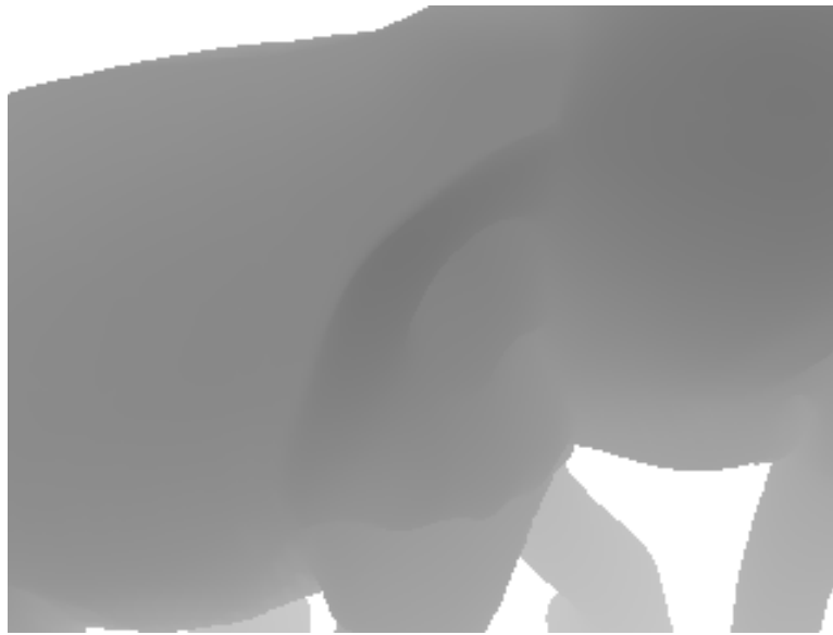
Figure 6-3: Ground-truth depth image of elephant model, from OpenGL z-buffer.
